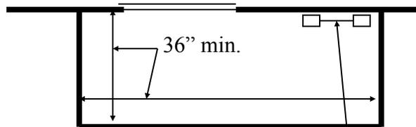
Ladder or stair permitted to encroach a maximum of 6 inches into required dimensions.
