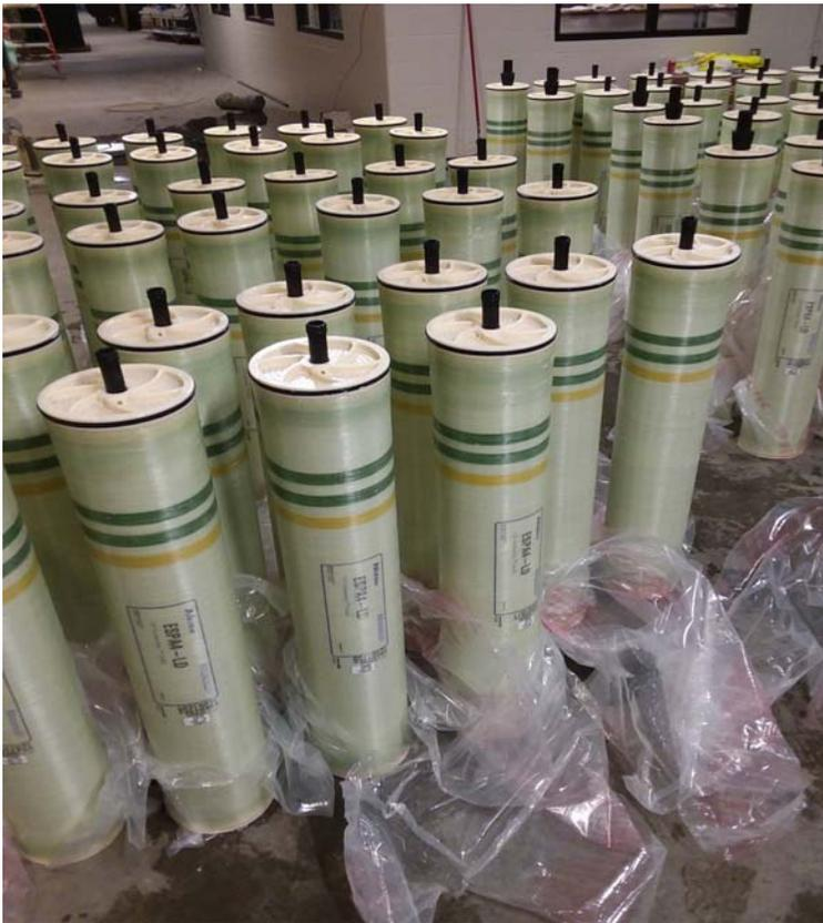
Hydranautics ESPA4-LD (low differential) Reverse Osmosis (RO) membranes elements being unpacked and prepped for installation.
