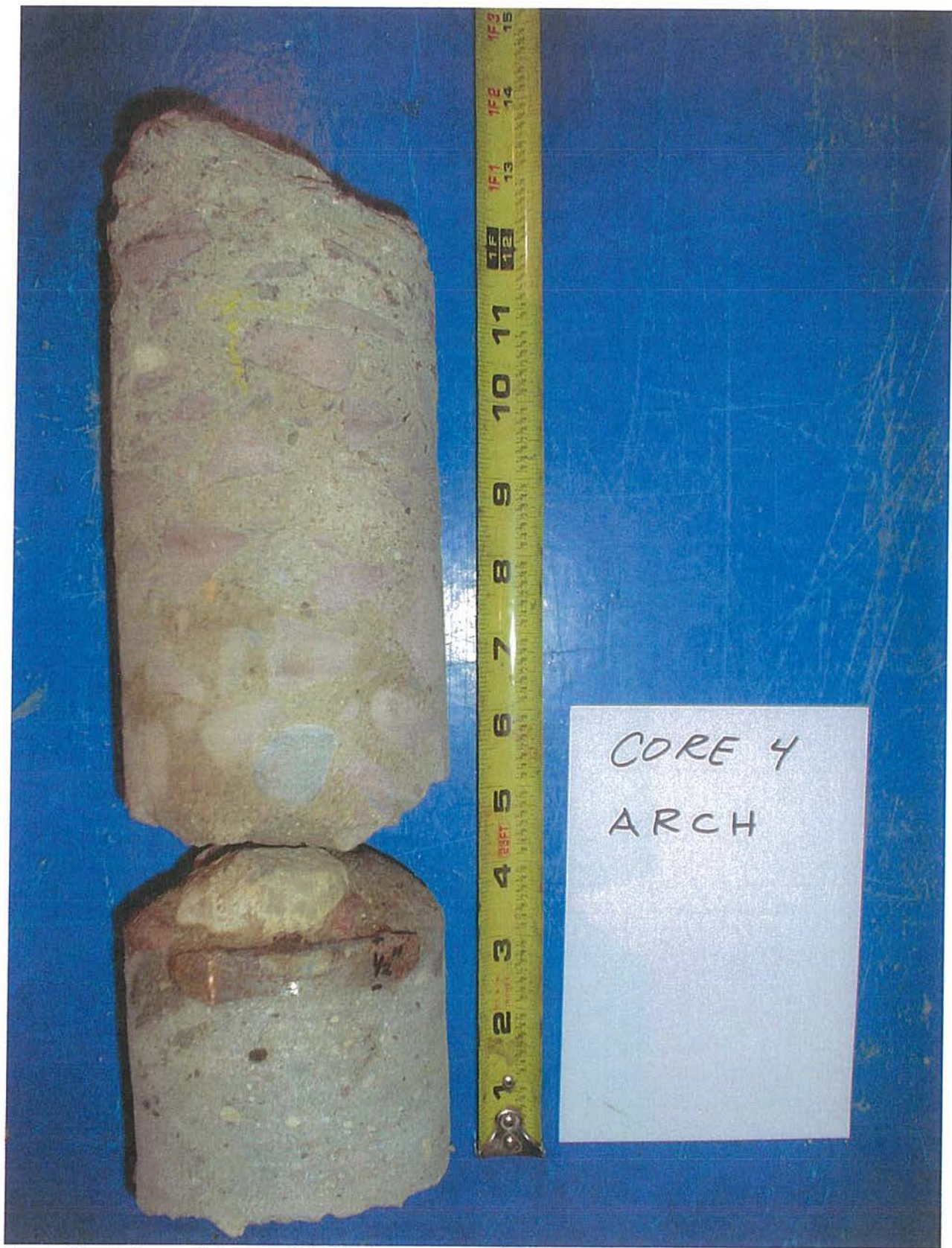
Image 30: Arch core 4 showing 1 1/2 inch aggregate and 1/2 inch steel reinforcement
