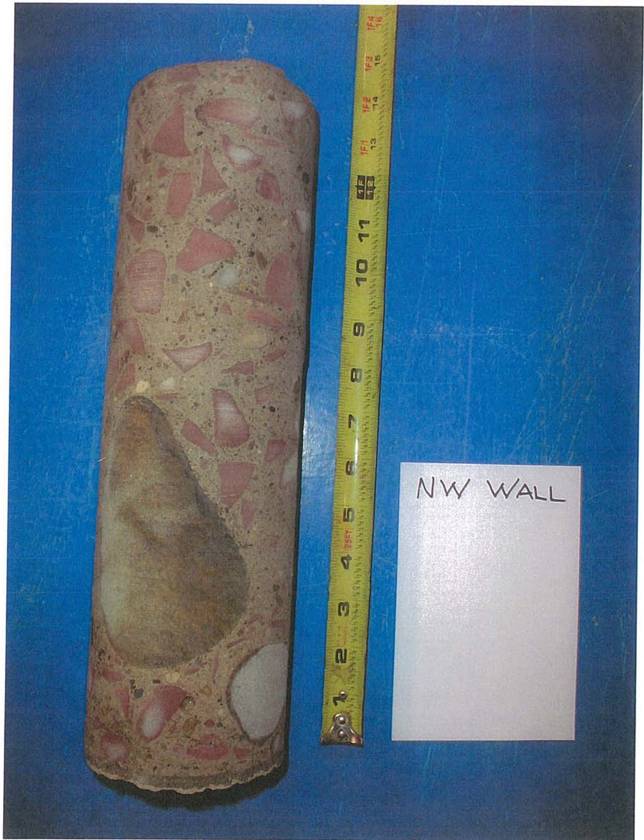
Image 18: Core sample from the northwest wall showing large aggregate
