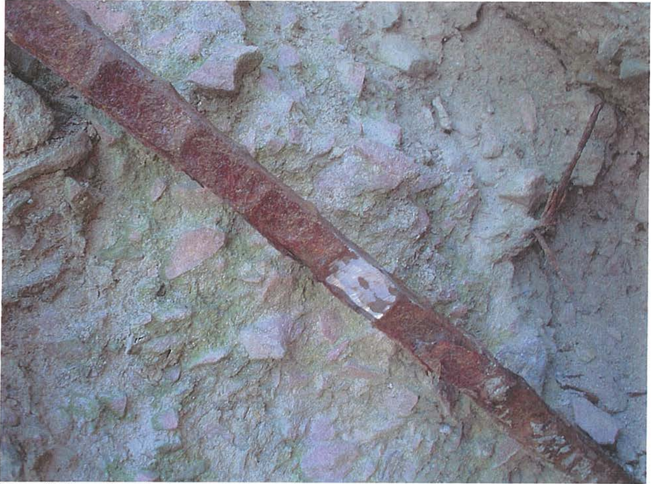
Image 10: Exposed steel reinforcement bar used to connect the voltmeter during the corrosion potential survey. Image shows the bar after grinding the corrosion from the surface of the bar.
