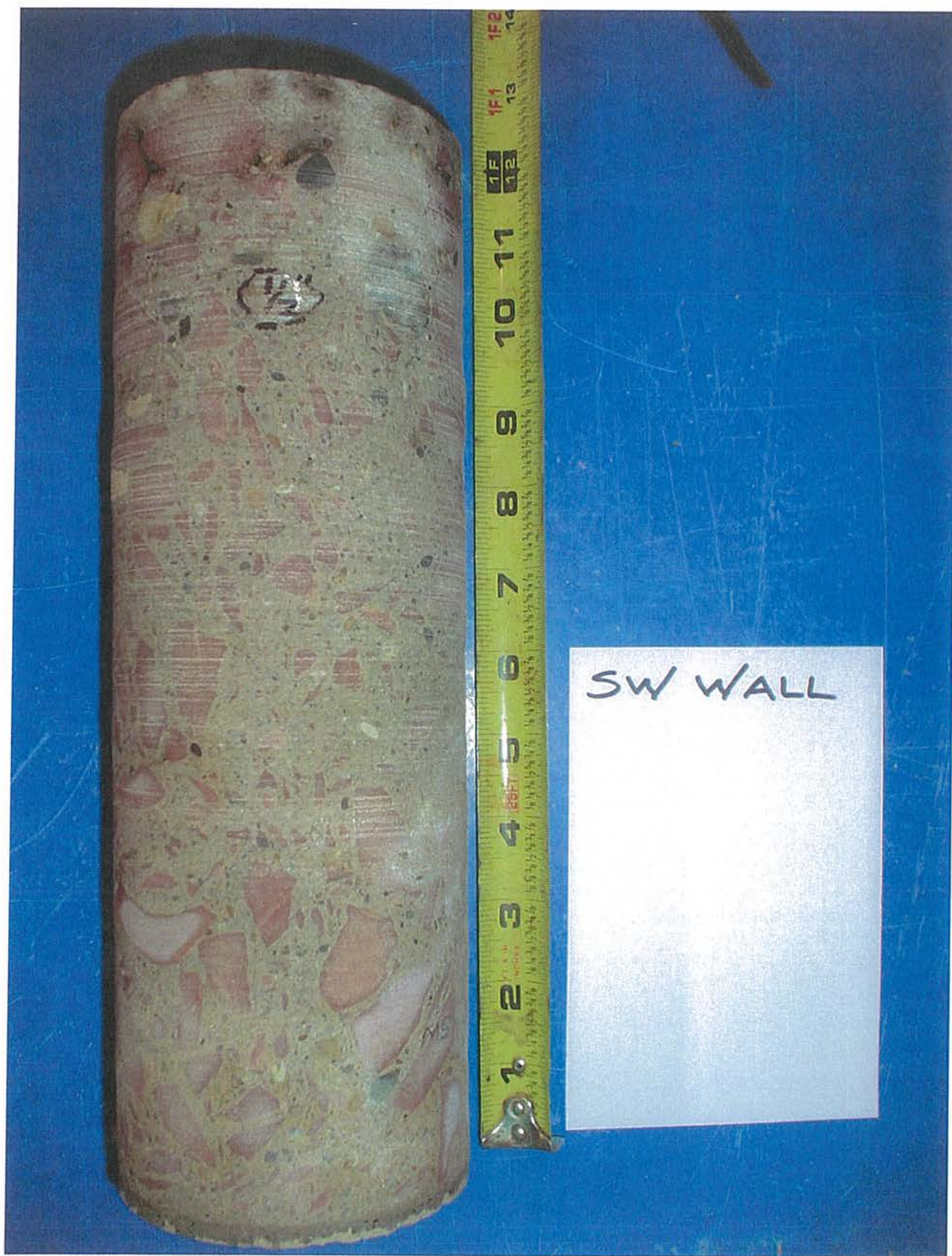
Image 16: Core sample from the southwest wall
