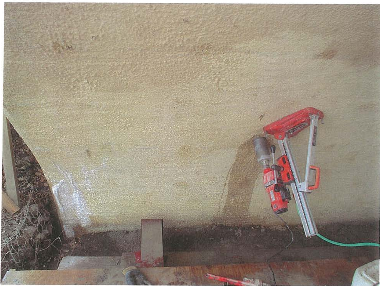
Image 33: Location of arch core 7 with core drill mounted to arch
