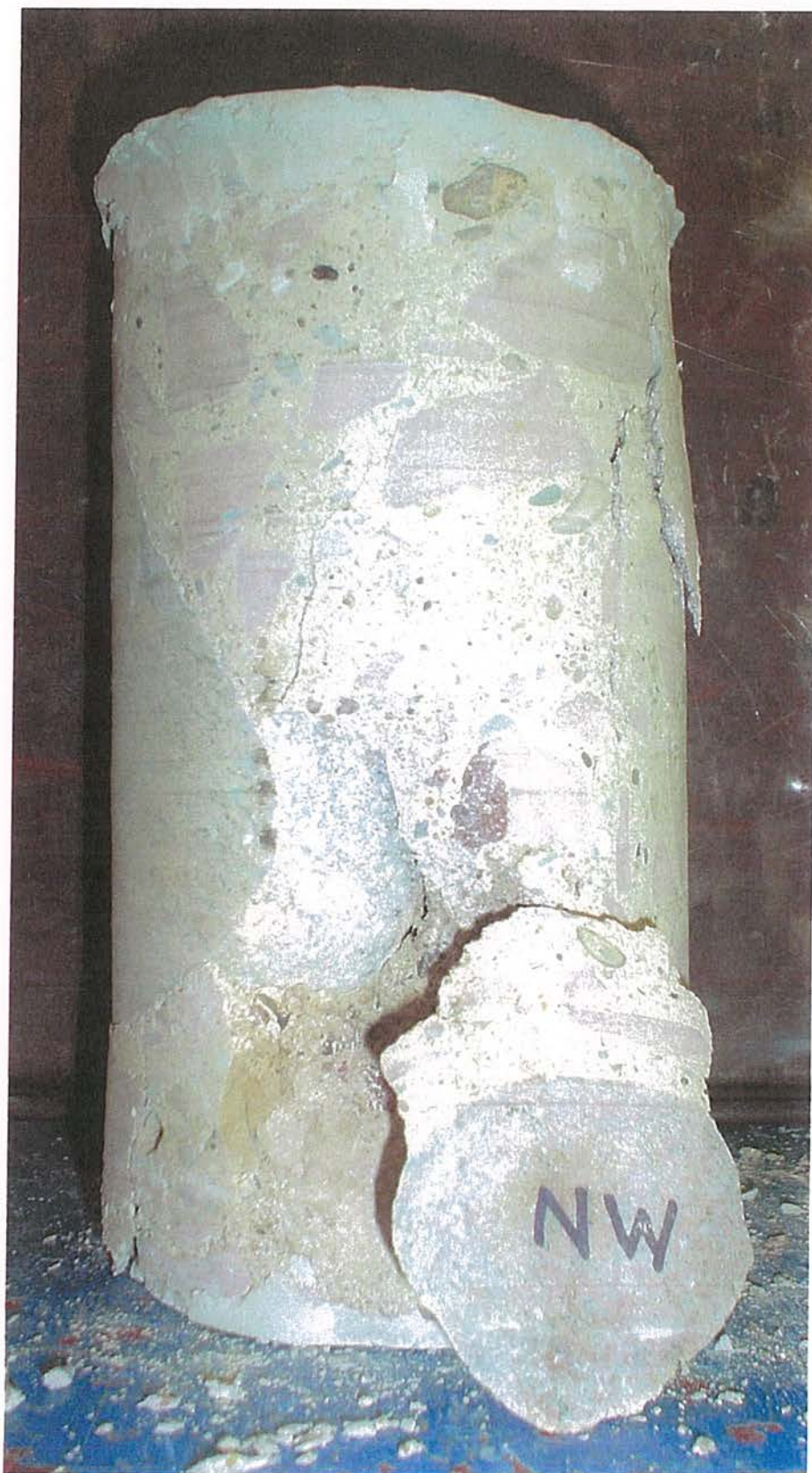
Image 20: Core sample from northwest wall after compressive strength testing
