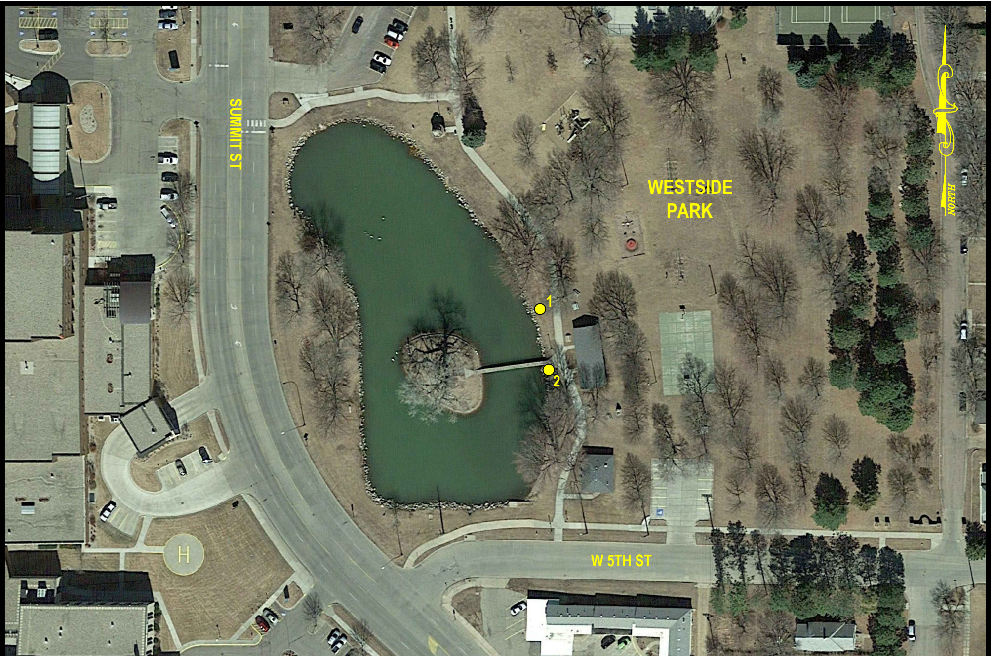
FIGURE 2 TEST BORING LOCATION MAP PROPOSED PEDESTRIAN BRIDGE & RETAINING WALL WEST 5TH STREET & SUMMIT STREET YANKTON, SD ACAD/GEOTEK/NICK/22-070
